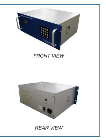
This matrix system consists of two 4x32 switching systems in a 4U standard 19" chassis. This switching system has an operating frequency range of 2-4GHz (S-Band). The output ports are internally terminated to  $50\Omega$ , controlled via USB and feature 7-segment displays which let the user know which output is currently active. There is also a local control keypad that allows users to manually command the switching system.
