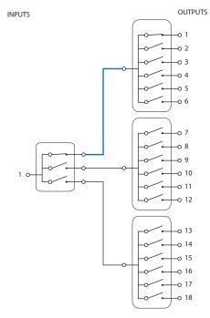
The multiplexor is the simplest matrix configuration, allowing the input to be connected to any one output at a time. Before switching, for example, to Output 2 the connection to Output 1 needs to be disconnected.
