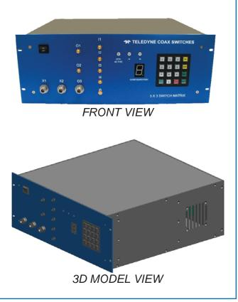
This matrix system consists of a 1x32 switching system with 2 bypass paths in a 4U standard 19" chassis. This switching system was designed for an operating frequency range of 2-4GHz (S-Band). The input and outputs are internally terminated to  $50\Omega$ , controlled via Ethernet port and feature 7-segment displays which let the user know which output is currently active. There is also a local control keypad that allows users to manually command the switching system.
