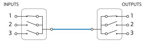
In a MIMO Single Connection Matrix, you can have Input 1 connected to Output 3, but you must disconnect this path if you were to connect Input 2 to Output 1, or any other combination.
