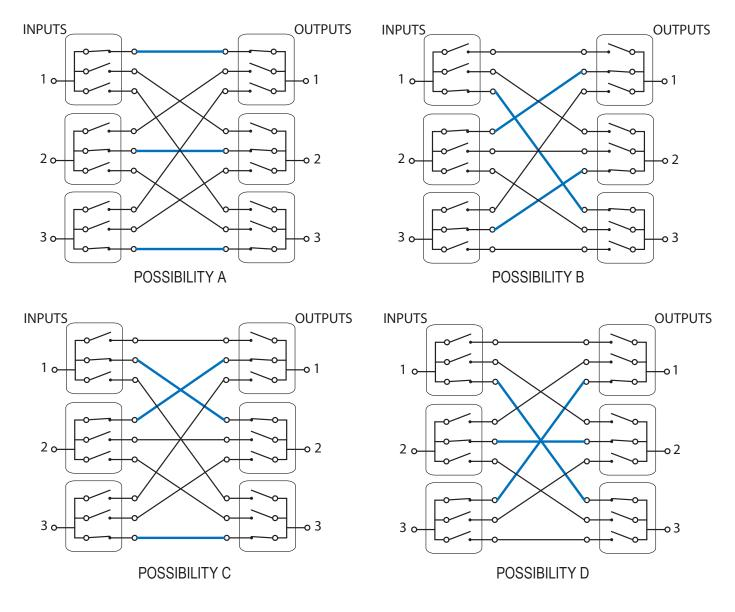
This matrix type, while being multiple-input, multiple-output, will allow a single connnection from any input to any output at a time. This means that the user can have (as shown in "Possibility B" Input 1 connected to Output 2, Input 2 connected to Output 1, and Input 3 connected to Output 3, all at the same time. The configuration shown would use 6 SP6T coaxial switches to create 9 distinct switch paths.
